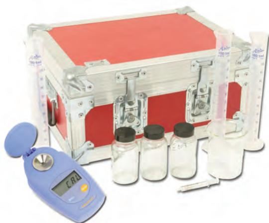
This Produced Foam Test Kit enables foam induction systems to be easily calibrated. Each kit contains a step by step manual together with worked examples.
